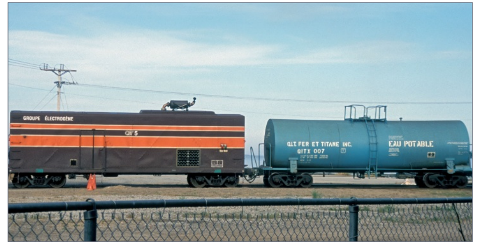
22. The blue tank car at right carries potable water. It and other cars hauling non-hazardous materials generally move with passenger trains. At left is a HEP generator car for the passenger coaches.
