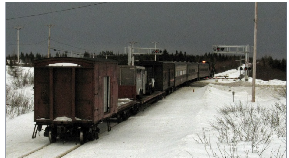
23. MP15 no. 10 leads a southbound QIT passenger train to Havre St. Pierre. Traveling with the coaches are a HEP genset, a flatcar with a truck, and a work service car.
