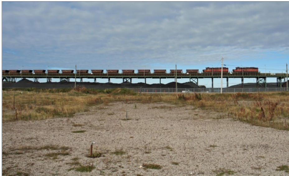
13. QIT GP9 27 and 40 unload ore cars on the ore dock at Havre St. Pierre. Half the train is unloaded at a time on the dock, with the ore dumped through the bottom.
