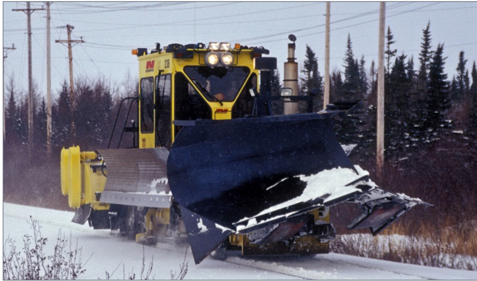
24. QIT uses this self-propelled snowplow to keep its line open. Previously, the railroad used snow-clearing trains with Russel snowplows.
