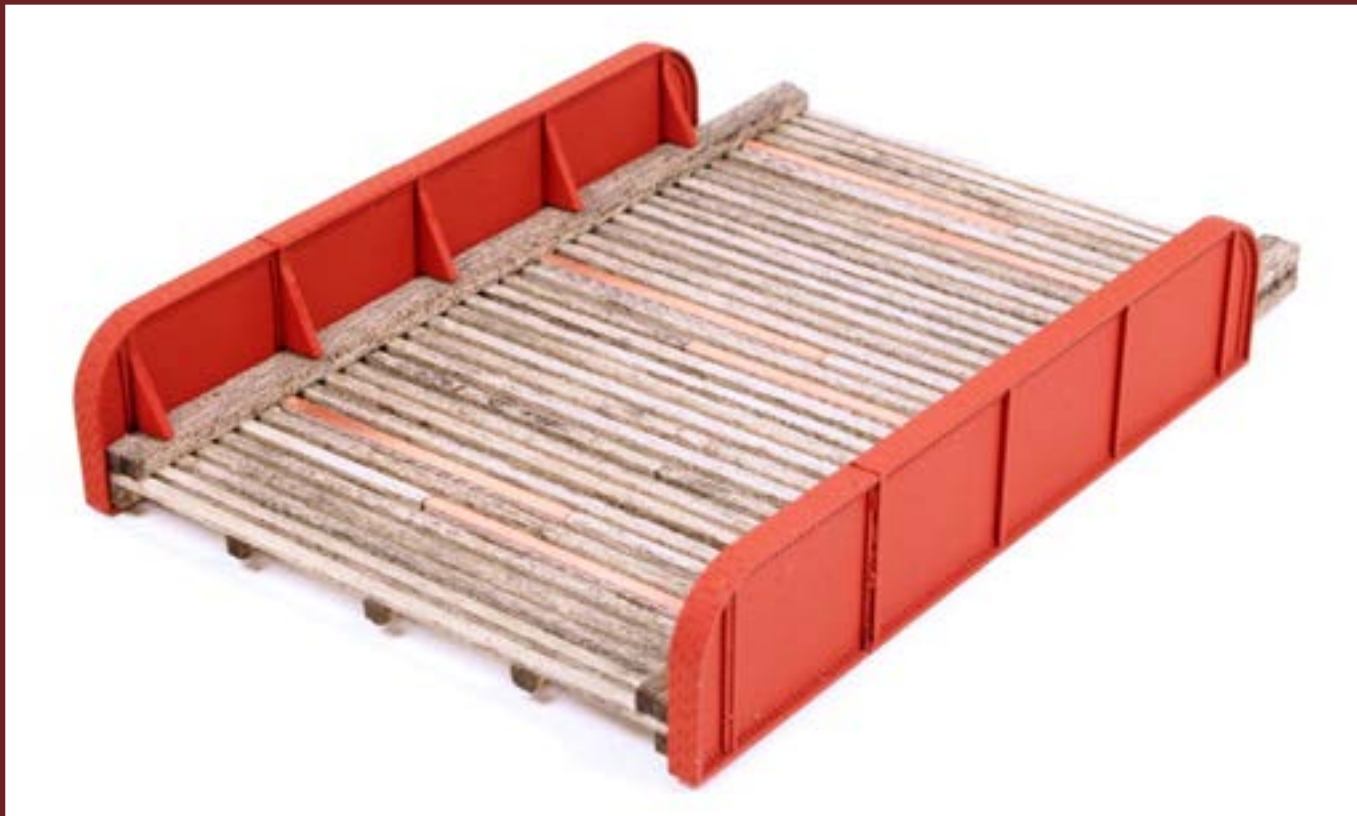
Figure 11: PC board ties, spaced out every \frac{3}{4} " or so between the \frac{1}{32} " x \frac{3}{64} " basswood boards, provide a secure place to solder the barge rail to the apron deck.
