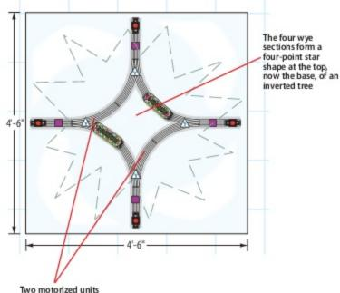
can bounce between two of the four points. With a proper type of train and switch control device, you can also have a single unit bounce between all four points
