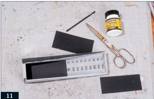
11 Window glazing and view blocks complete the interior.
