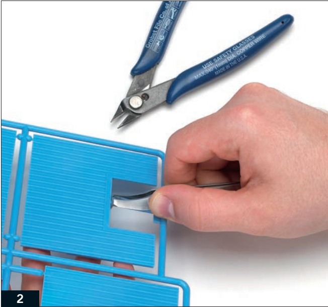
2 Remove parts from their sprues with sprue-cutting nippers (from Micro-Mark and others) or flush cutters.
