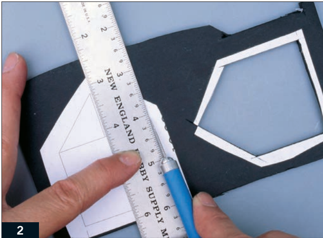
2 To make assembly of the foam core walls easier, hold the hobby knife (with a new, sharp blade) so that the cut edges are 90 degrees to the surface.
