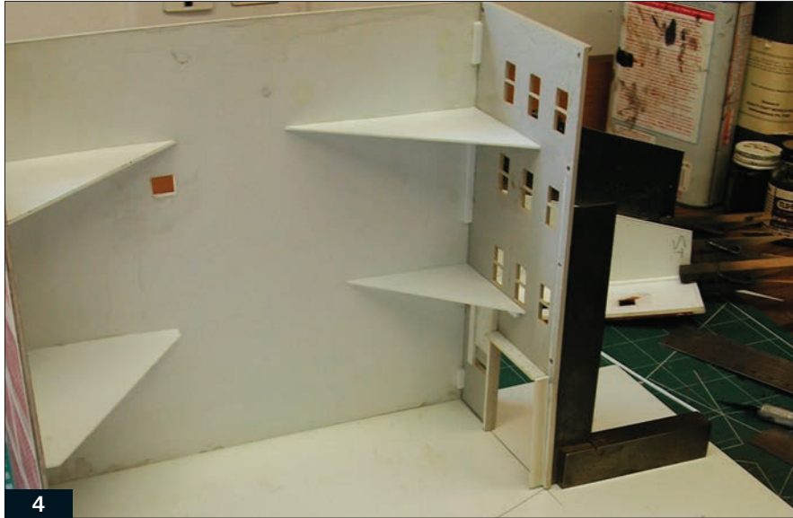
4 I assembled and braced the corners of all three straight walls before determining the final outline of the styrene roof.
