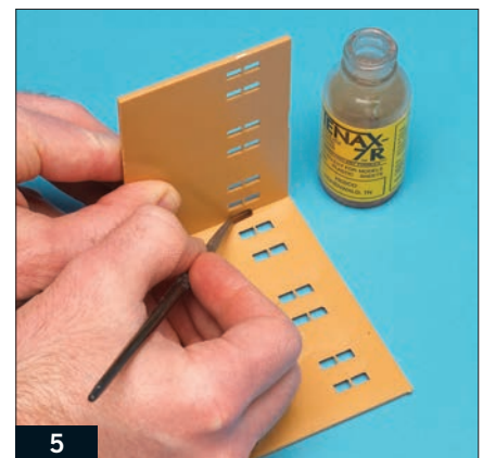
Touch a brush of liquid plastic cement to the joint and capillary action will draw it into the seam. Hold the joint securely for a few seconds until the bond begins to strengthen.
