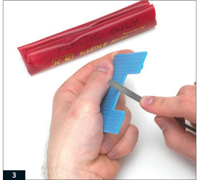
3 Use needle files to smooth any flash or rough areas from sprue-connection points.
