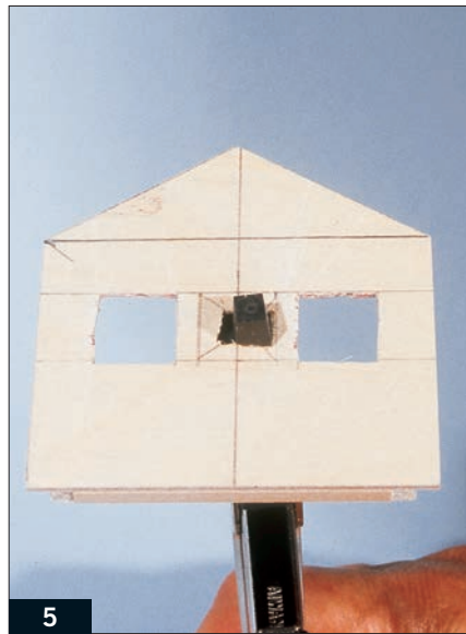
I used a nibbler, a tool designed to cut openings in electronics cabinets and panels, to cut out the windows in the station's plywood walls.
