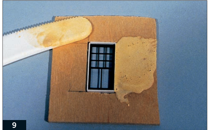
9 To simulate stucco, spread a thin layer of Durham's Water Putty with a plastic knife. It's easy to spread right up to the window and door casings.
