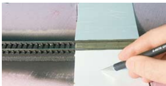
Fig. 3 Adding cracks and joints. Use a sharp hobby knife to scribe expansion joints and cracks into the surface of the road. Don't get too carried away with this step!
