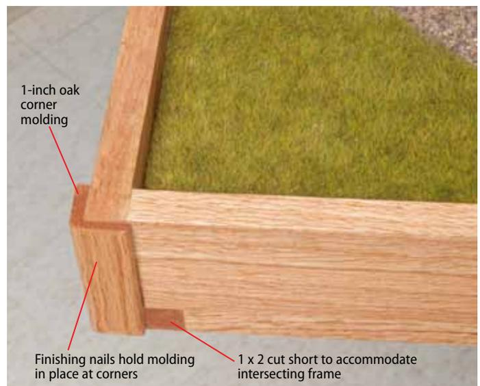
After allowing the glue application along the framework and corners to dry, we decided to add finishing trim to each corner. We cut four 3/4-inch lengths of outside corner molding for the corners and attached them with carpenter's wood glue. You can use small finishing nails to hold them in place if you wish, but be sure to drill pilot holes first and fill the nail holes afterward.
