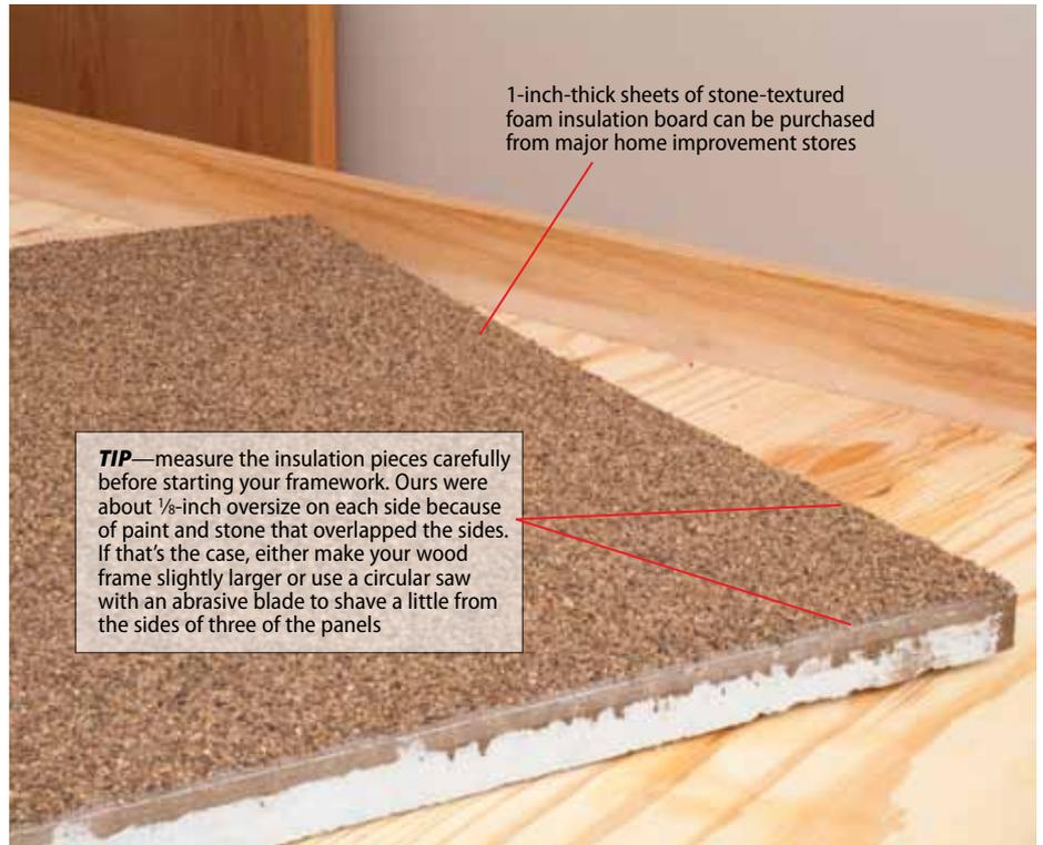
On our project layout, the 2 x 4-foot sheets of stone-covered insulating material add strength to the plywood. Plus, in our application, it saved a lot of time because it allowed us to skip ballasting completely—something we really didn't miss!
