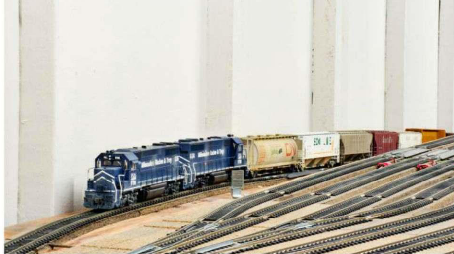
Without the vertical curve at the crest of this grade in the staging area of Model Railroader's club layout, couplers would separate at the kink. Bill Zuback photo
