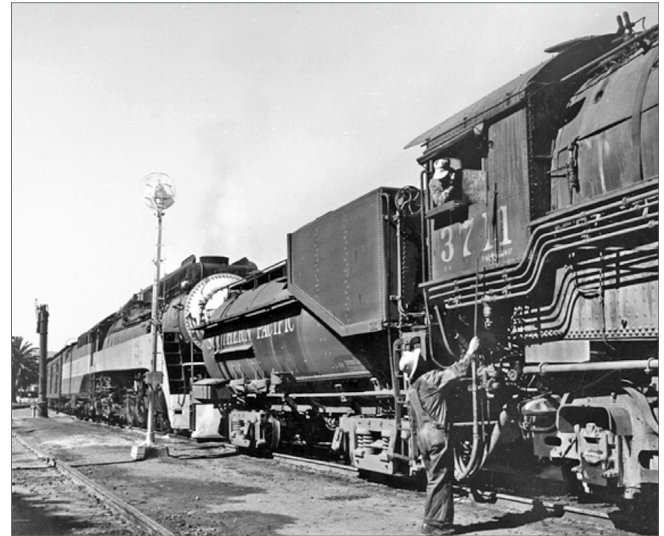
20. In this photo at San Luis Obispo, 2-10-2 helper no. 3711 is about to help the westward Daylight, no. 99, over Cuesta. The engines are coupled up and all servicing has been completed, so the worker on the ground is about to remove the metal blue flag from its place on the cab side (just to the right of the engineer). The flag reads "MEN AT WORK," and Rule 26 provided that it be placed on engineer's cab side. Richard Steinheimer photo, De Golyer Library
