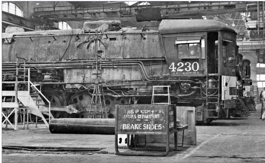
16. This 1955 view inside the Erecting Hall at Sacramento General Shops shows cab-forwards undergoing class repairs. In the foreground is a skid for brake shoes, labeled "SP CO STORES DEPARTMENT," as well as indicating the desired contents. Ken Yeo photo, Bob Church collection
