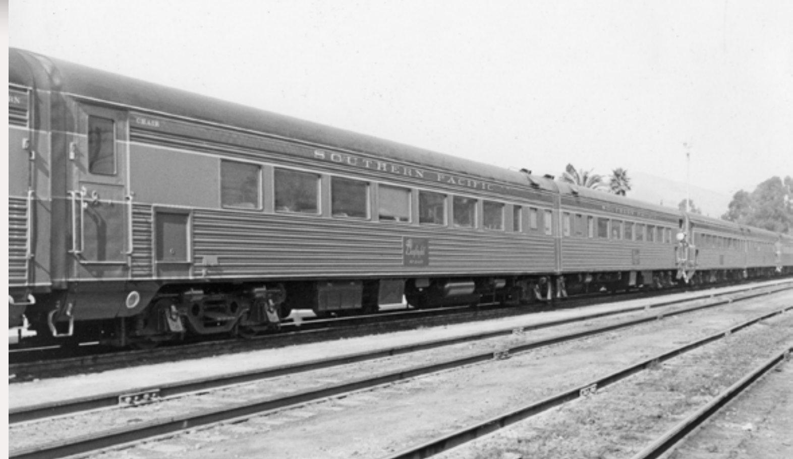
Figure 34: An articulated two unit chair car. The square recessed door next to the passenger entry is a dumbwaiter (also called a baggage elevator), it permits quick loading of passenger carry-ons without blocking vestibule steps at stations. The photo can be dated in the mid fifties – the car is still in Daylight colors but already has its skirting removed - photo courtesy Bob's Photos .
