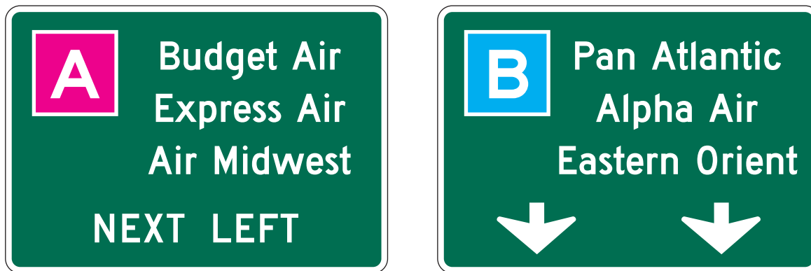
Figure 2D-1. Examples of Color-Coded Destination Guide Signs
