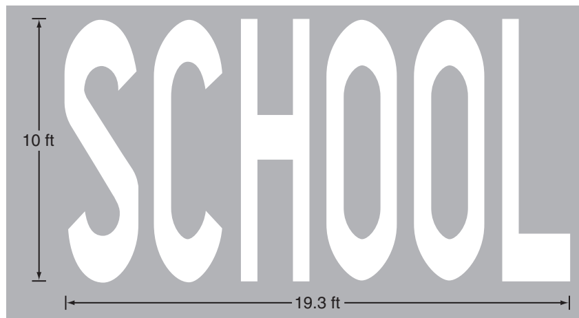
Figure 7C-1. Two-Lane Pavement Marking of “SCHOOL”
