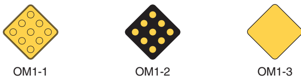
Type 1 Object Markers (obstructions within the roadway)
