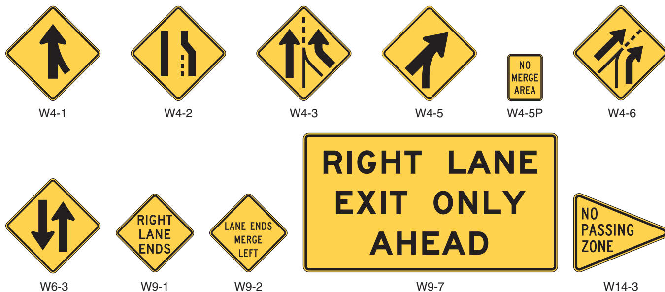
Figure 2C-8. Merging and Passing Signs and Plaques
