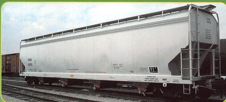
CCBX 58792 is part of the new generation of “high-cube” plastics cars. This one was built by Thrall in 1995. It has a 6,270 cu.ft. capacity. GRL is 286,000 lbs. (110-ton nominal).
