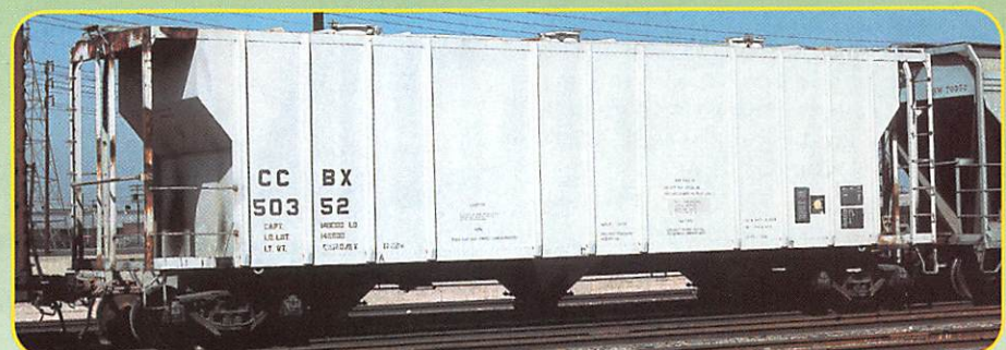
CCBX 50352 was built in November 1962 by Pullman-Standard. Rated at 3,520 cu.ft. — it's one of the first designs used for plastics transport. Seen here, in service, during August 1985. CCBX is Union Carbide.
