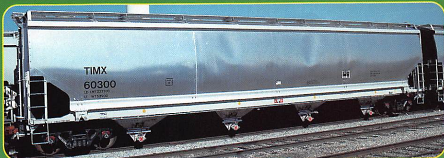
TIMX 60300 is a 6,011 cu.ft. capacity aluminum-bodied covered hopper for plastics service. In addition to being lighter, aluminum-bodied cars don't need to be lined. This car was built by Trinity Industries in 1998. So far there have been several hundred of these built. A very distinctive model this would be!
