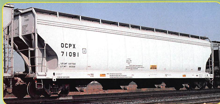
OCPX 71091 is a more contemporary version of ACF's 5,800 cu.ft. design. This one was built in 1994. There are a number of production variations (many subtle) in ACF's 5800s. OCPX is Occidental Chemical Corporation.
