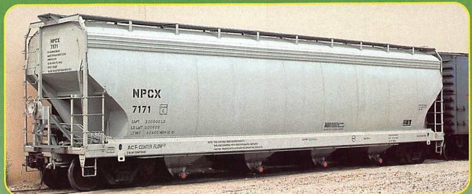
NPCX 7171 is a 5,400 cu.ft. design that was built in December 1981 (notice how many different designs were being offered in 1981 from ACF!). NPCX is currently a reporting mark of Equistar Chemicals, LP.
