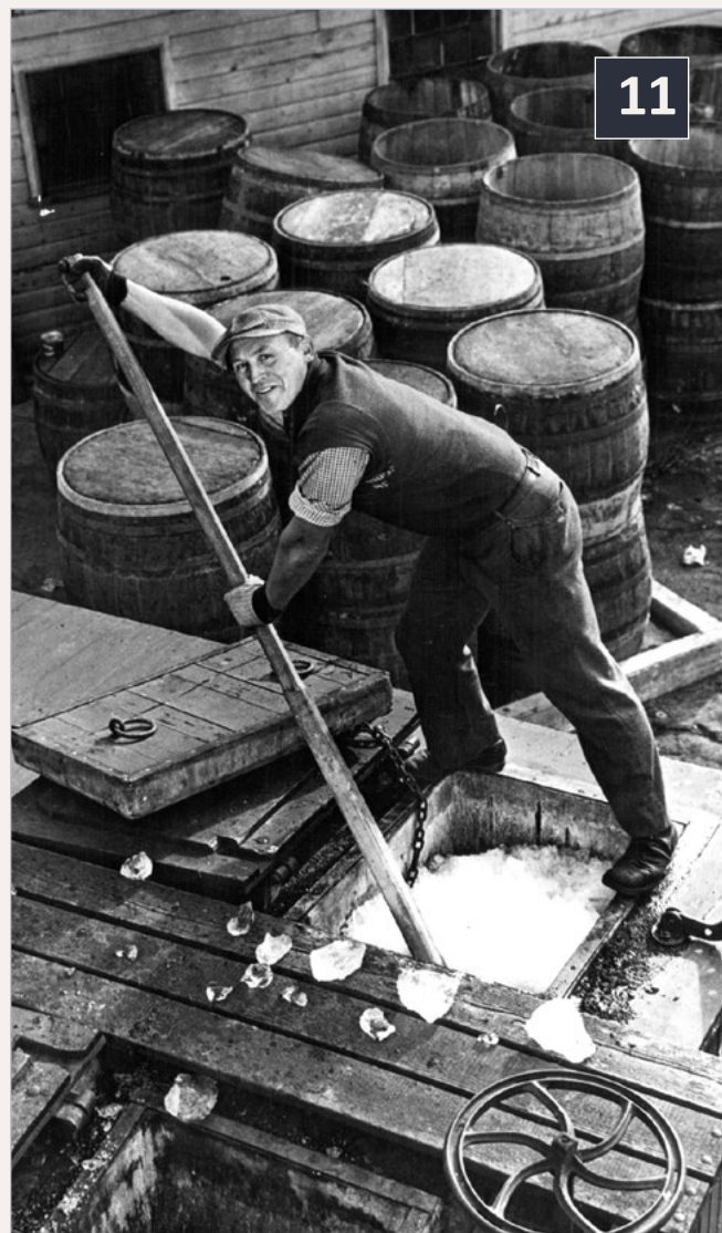
11: This workman is “bar-ring” the ice in the bunker. Ice size appears to be “crushed.” This is a Union Refrigerator Transit (URTX) car. Note the separate hatch plug, of canvas-covered wood construction, lying atop the hatch cover. – Arnold Menke collection.
