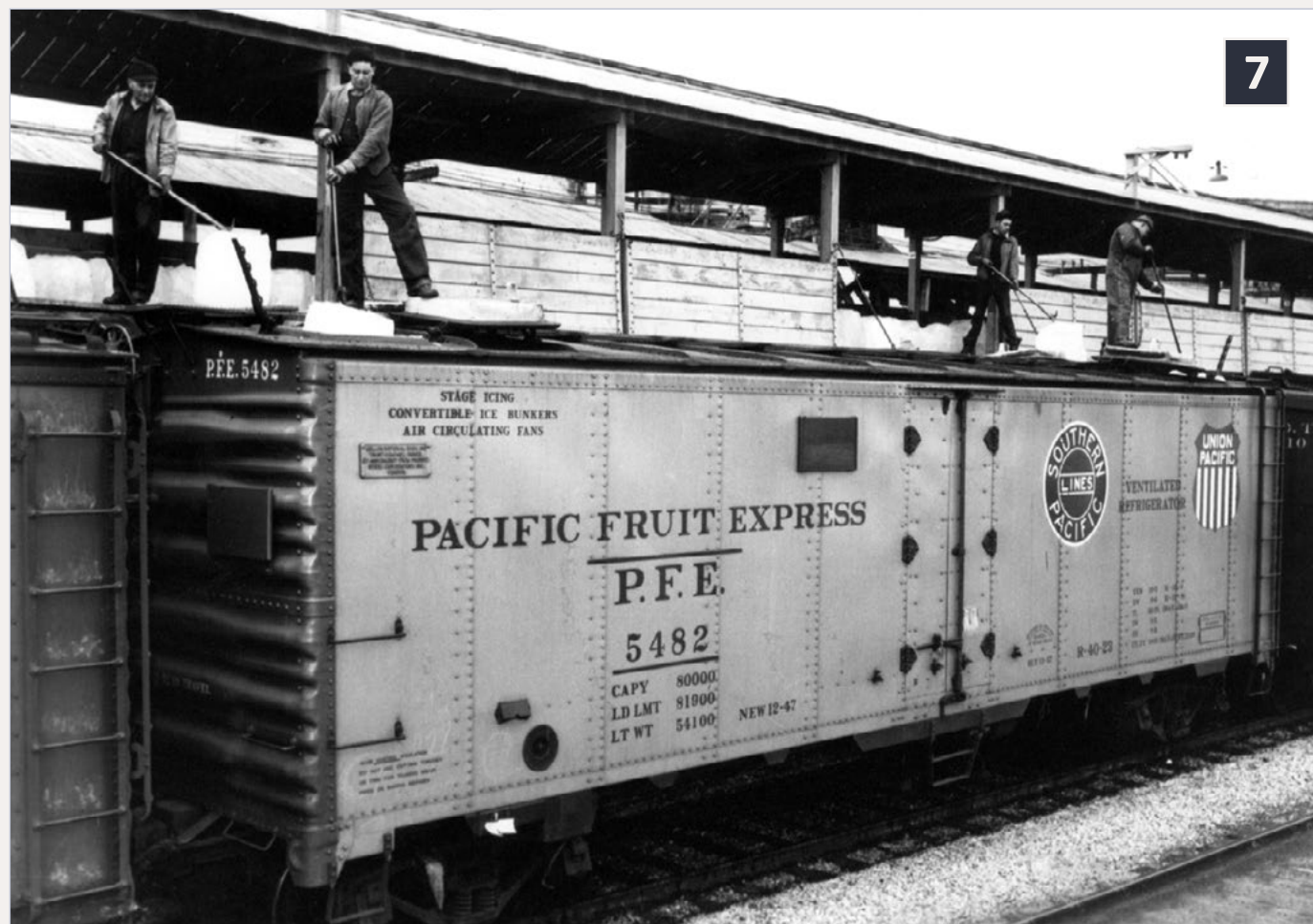
7: In this photo, the typical two-man crews are doing much the same job as in the Morley photo, though in this case with a steel car of Class R-40-23. –PFE photo, courtesy CSRM
