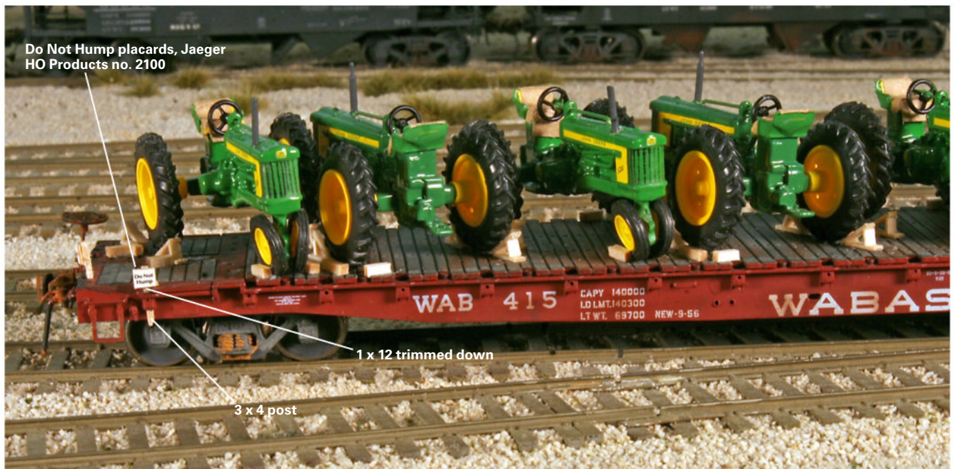
Fig. 5 Safe handling. These DO NOT HUMP signs alert train crews not to route this car through a hump yard. Mont made the signs using trimmed down 1 x 12 and 3 x 4 stripwood.
