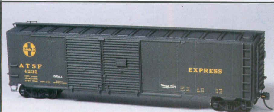
Mike modified a Life-Like Proto 2000 50-foot box car kit with, among other minor changes, passenger train air, signal, and steam lines like those in Cal Scale's 275 set.
