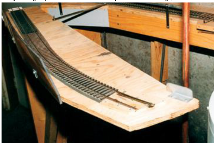
Photo 4 — Closeup of top hinge and draped power wire.
