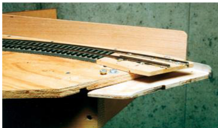
Photo 1 — The docking section contains a lip to accept the gate. You can see a stop made from a piece of 1" x 1" aluminum angle. The gate slips between the lower lip and the one made of basswood where rails are attached.
