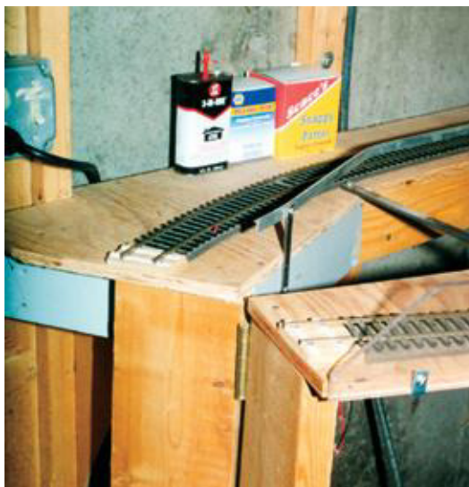
Photo 3 — The hinge side made from 2 x 6 framing lumber
