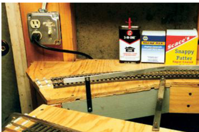
Photos 6 and 7 — Traingate open and tucked away showing retaining bar and guardrails. Note that benchwork also becomes a catchall for sundry household items – some typical, some questionable.
