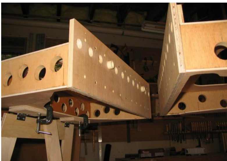
This photo shows two of the modules Jerry was building in the early stages of construction. Note the torsion box construction and all the lightening holes. The scenery was to be made with light insulation foam to keep the weight down. The legs are Jerry's idea also. They are very simple to build and fold very flat for easy transporting.
