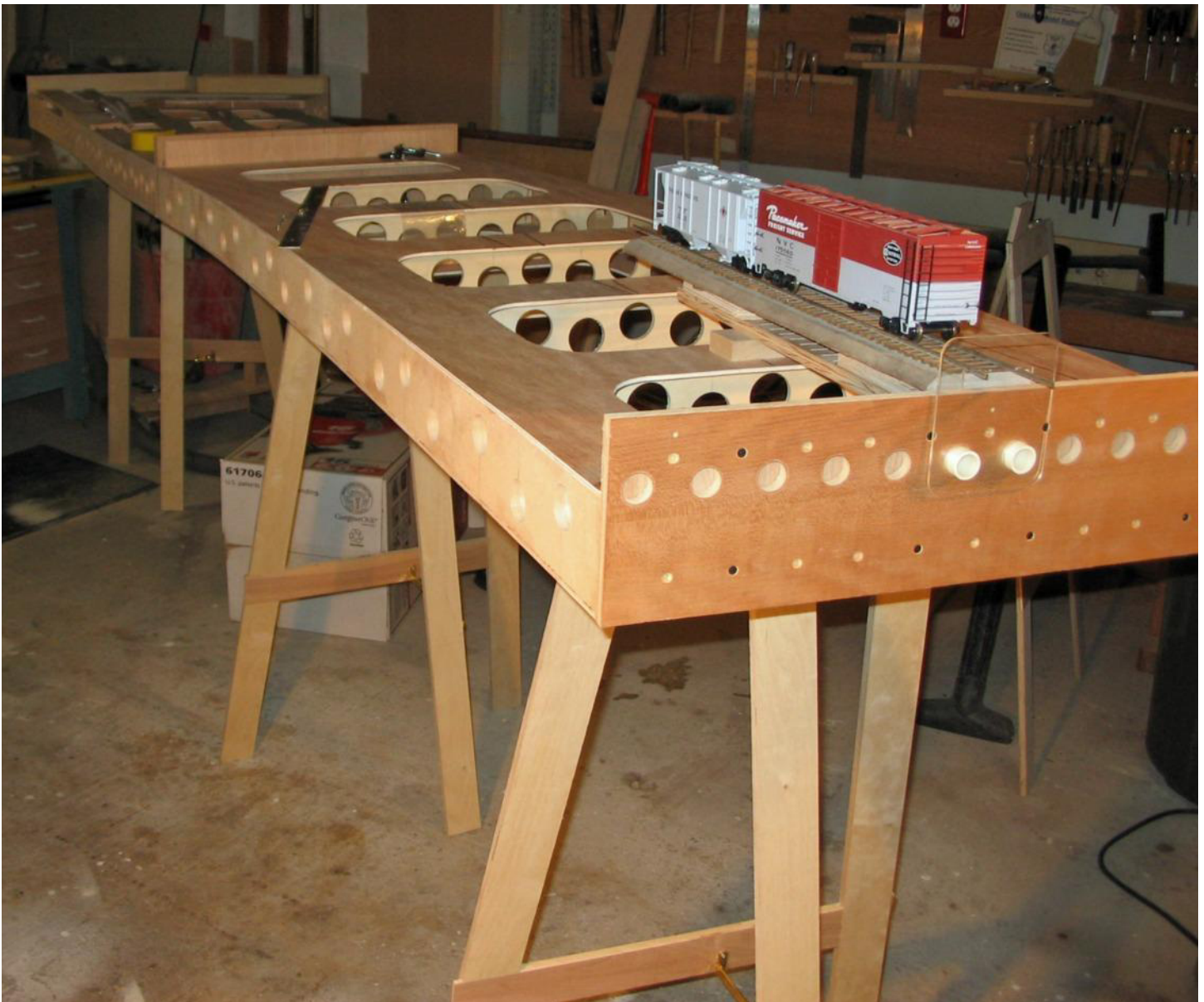
This photo shows two of the modules Jerry was building in the early stages of construction. Note the torsion box construction and all the lightening holes. The scenery was to be made with light insulation foam to keep the weight down. The legs are Jerry's idea also. They are very simple to build and fold very flat for easy transporting.
