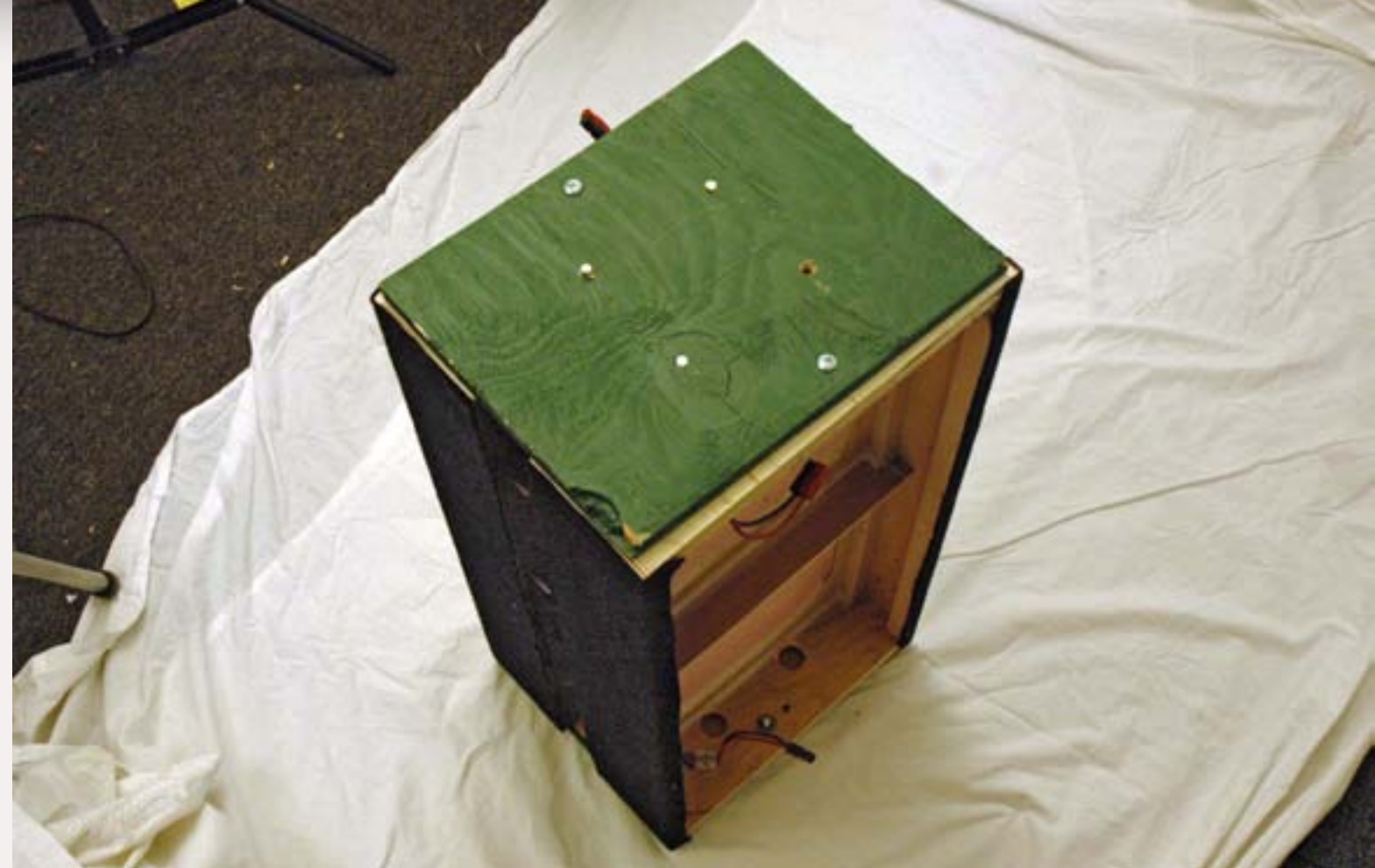
FIGURE 11: Green plywood endplates are used to hold two modules face to face for transportation. You can see the pins in their respective holes and the machine bolts holding everything together. This helps to avoid undue wear and tear on the modules viewing surface during the many hours spent in transit. No problems have been encountered with the loose electrical connectors during travel. These modules can be stacked like cordwood in a trailer or truck bed with little fear of damage. They are rugged, light and simple. Photo by Kevin Hunter.
