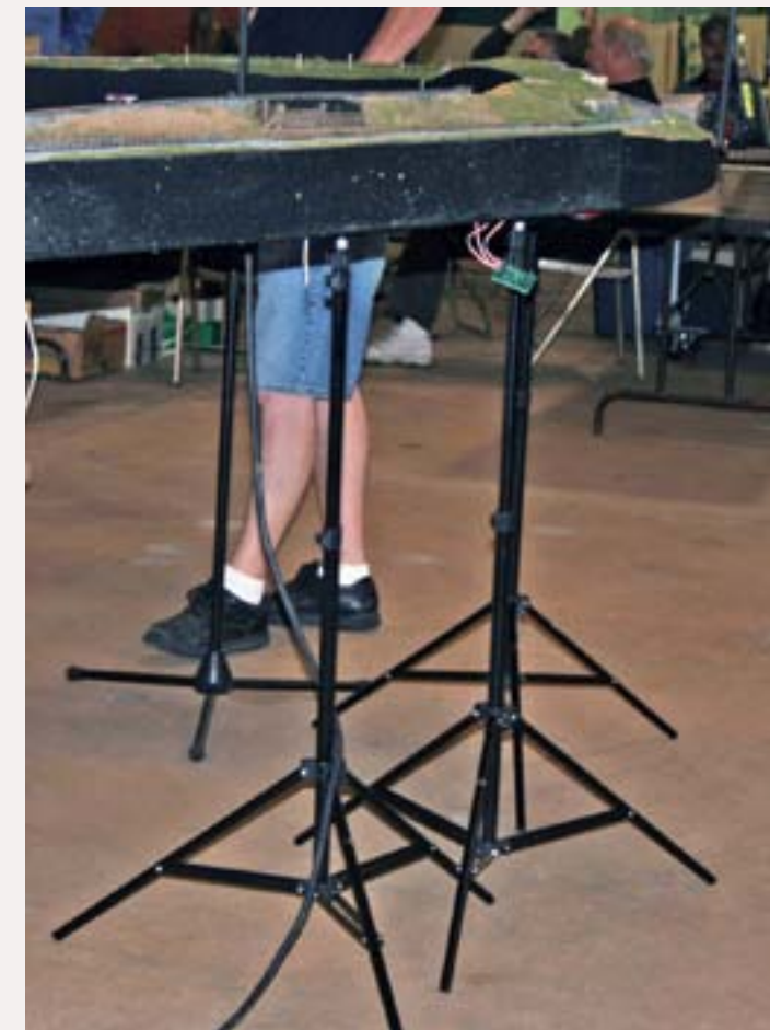
FIGURE 1: Each of the photographer's light stands (black legs) is supporting a module that is leveled along the rail and across the track. The white legs in the background are of a bipod module support that is only temporary and not nearly as strong.
